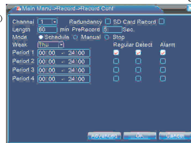
Picture 4.1 recording setup
