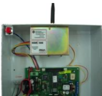
Figure 5. The GSM-200 installed in the control panel case (optional)
